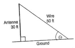
Find, to the nearest degree, the measure of the angle that the wire makes with the ground. [Show all work.]
